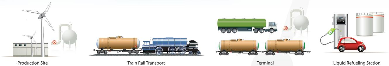
Figure 10. Pathway for Rail Delivery of Liquid Hydrogen
