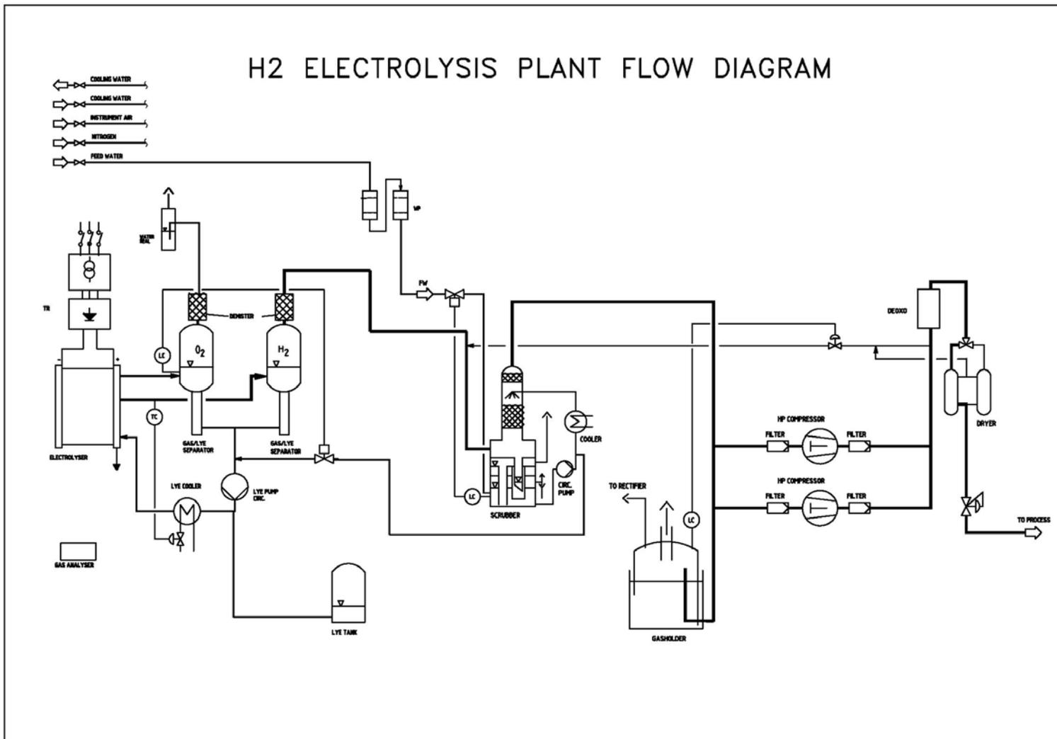
Figure 5.2.1. Distributed electrolysis process flow diagram (Ramsden, 2008b)
