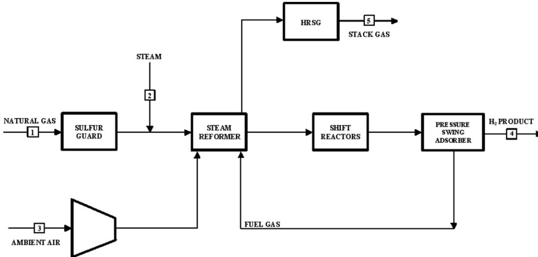
Figure 5.4.1. Central natural gas process flow diagram (Steward, 2008)
