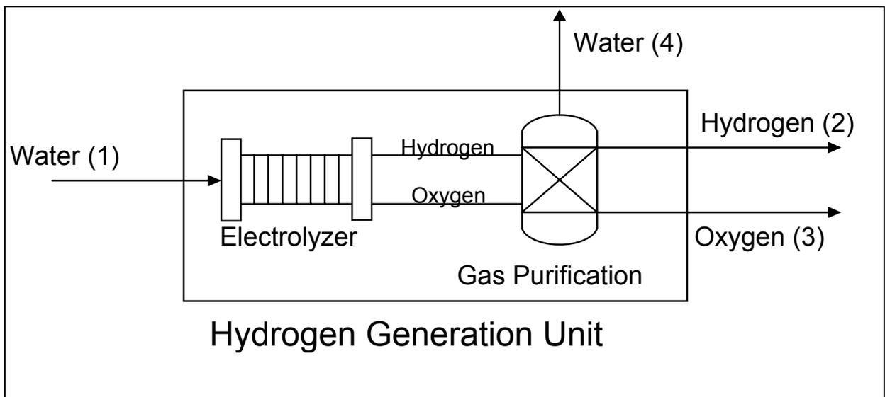
Figure 5.2.2. Distributed electrolysis mass balance diagram (Ramsden, 2008b)
