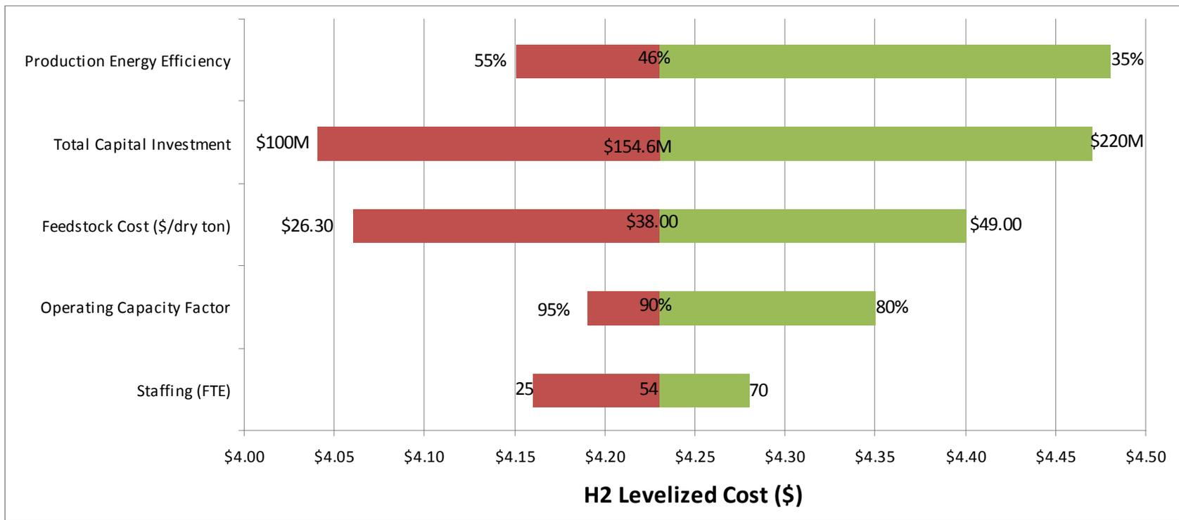
Figure 9.4.9. Production sensitivities for central biomass-pipeline delivery pathway
