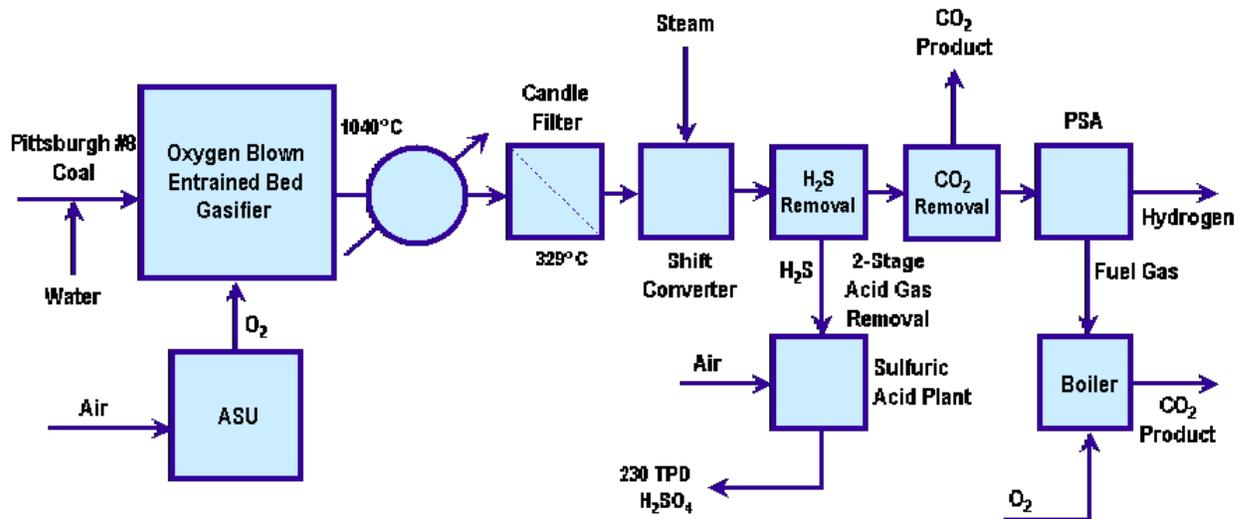
Figure 5.6.1. Central coal with carbon capture process flow diagram (Rutkowski, 2008a)
