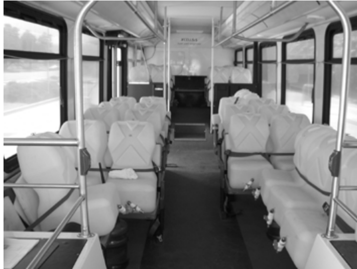
Figure 2. Water tanks in the XCELLSiS bus simulate curb weight during testing
