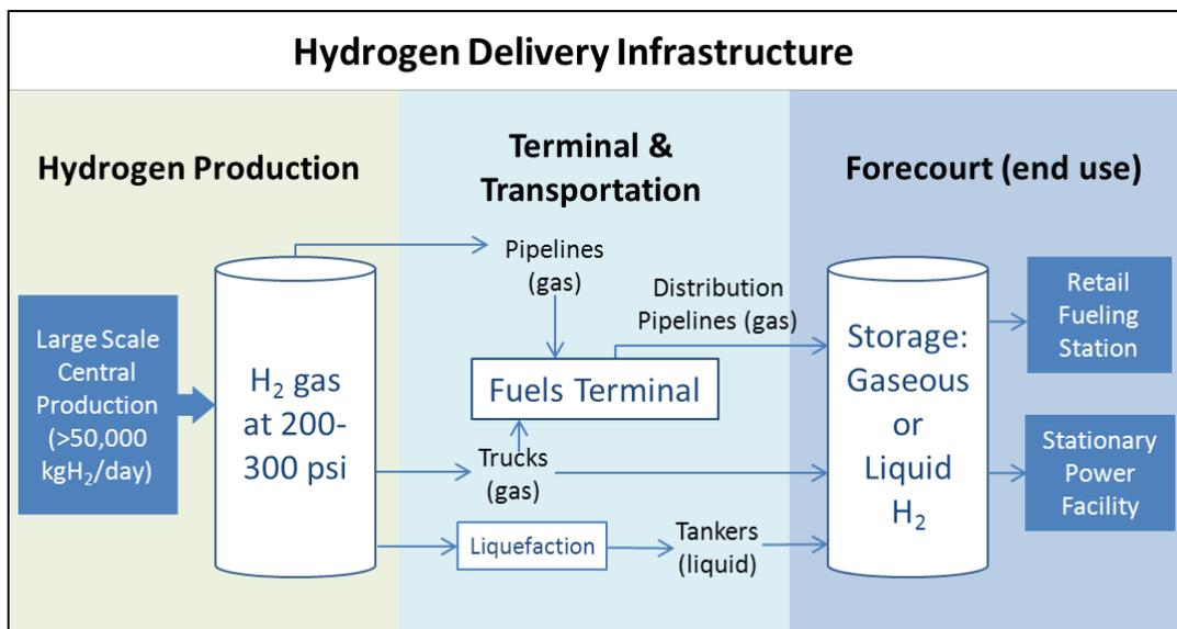
Figure 1. Hydrogen Delivery Scope
