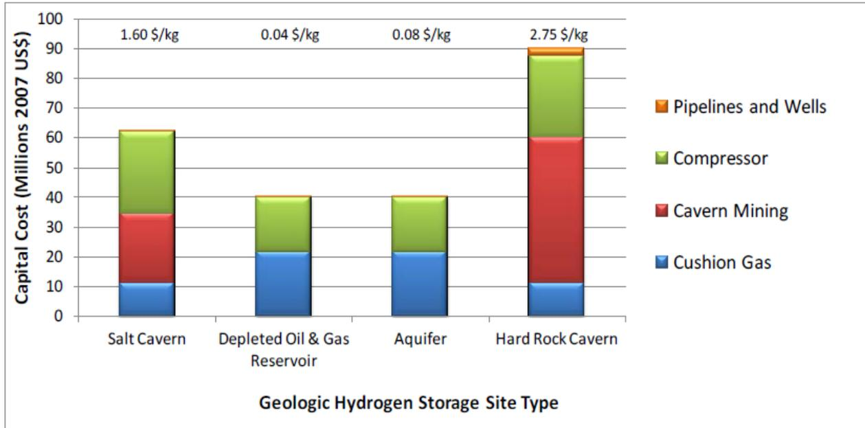
Figure 7. Cost Comparison of Geologic Storage Methods
