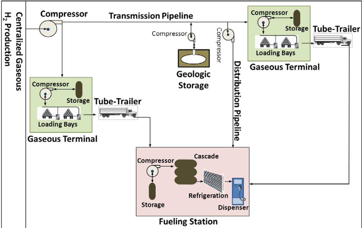
Figure 2. Example of Gaseous Delivery Pathway
