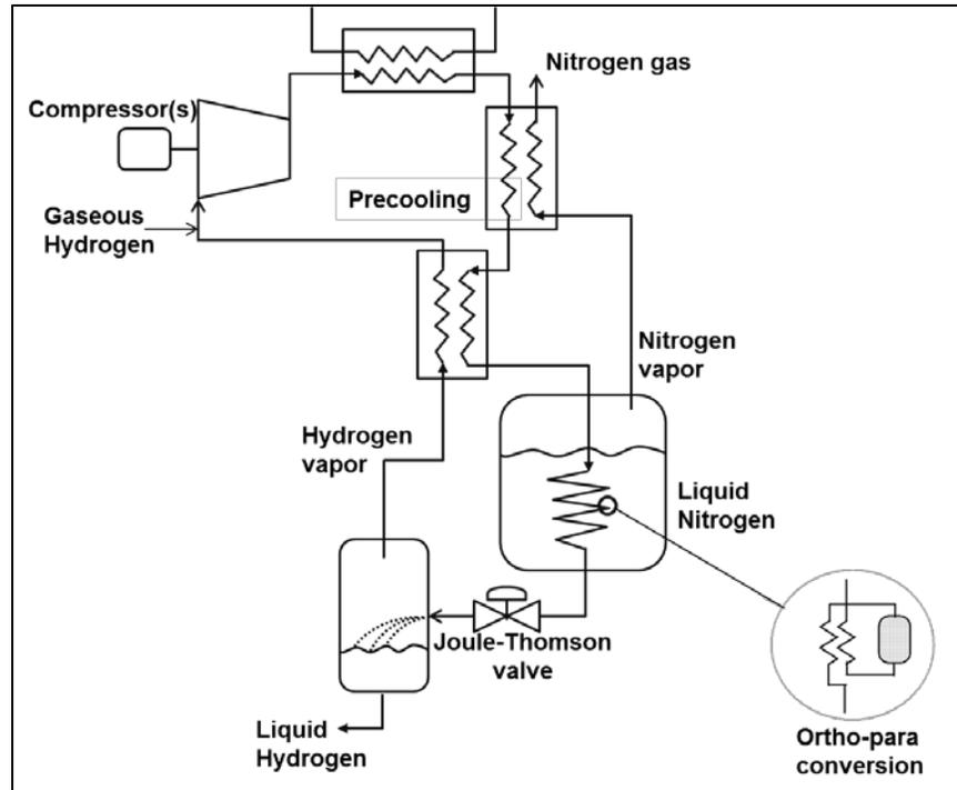
Figure 5. Hydrogen Liquefaction Plant
