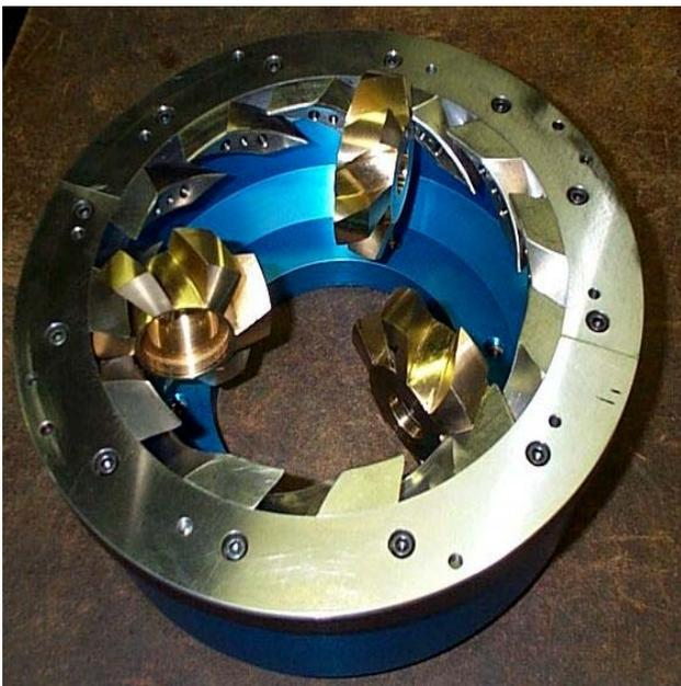
**Figure 3.** TIVM prototype compressor and expander vanes.
