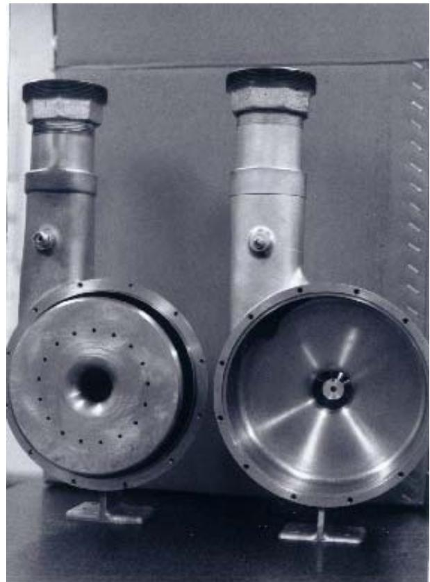
**Figure 4.** Meruit turbocompressor housings.
