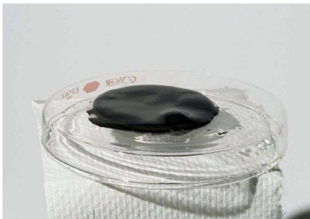
a. Hydrated bacterial cellulose after incubation in ammonium hexachloropalladate.
