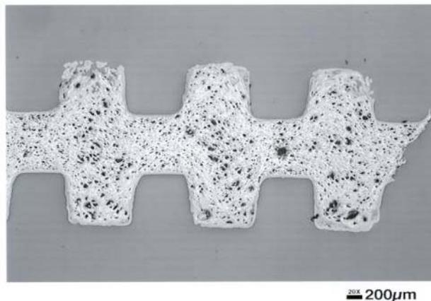
**Figure 2.** Optical micrograph of a polished cross-section of a carbon composite bipolar plate.
