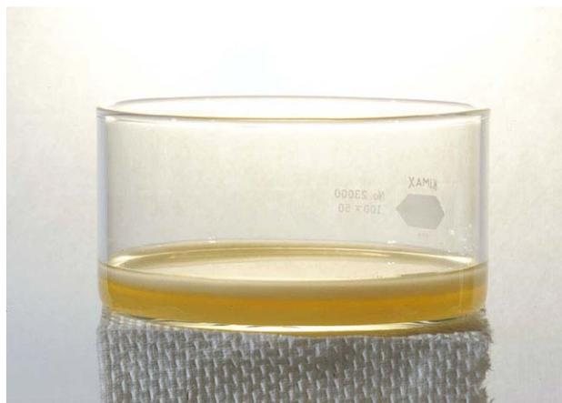
b. Processed bacterial cellulose after treatment with 1% NaOH and Na-acetate (pH 4.5).
