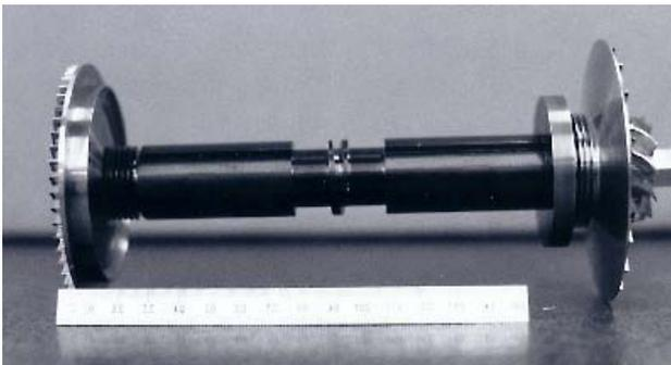
**Figure 2.** Meruit turbocompressor rotor.
