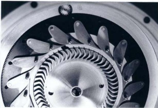
**Figure 1.** Meruit variable nozzle expander.
