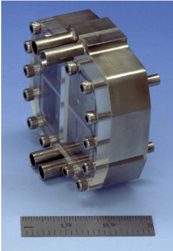
**Figure 1.** R&D 100 Award-winning microchannel gasoline vaporizer.
