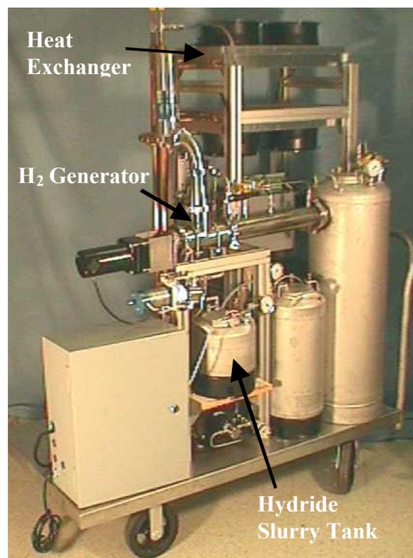
**Figure 2.** 50-kWe hydrogen generation system.
