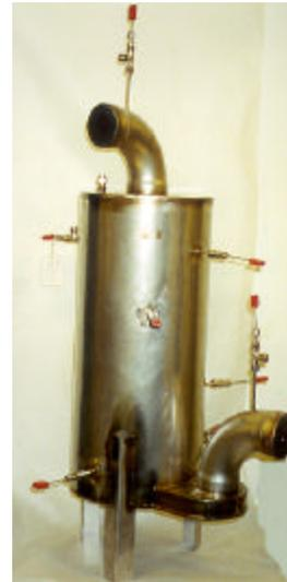
**Figure 2.** Low-temperature shift converter test article.
