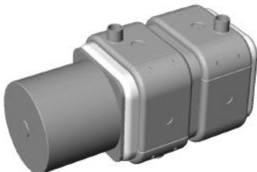
**Figure 8.** Motor/compressor/expander integrated for testing.
