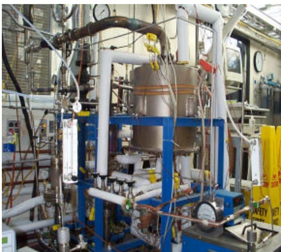
Figure 1. Model B fuel processor.
