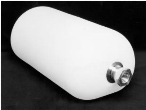
**Figure 2.** Full-scale plastic liner with aluminum polar boss.
