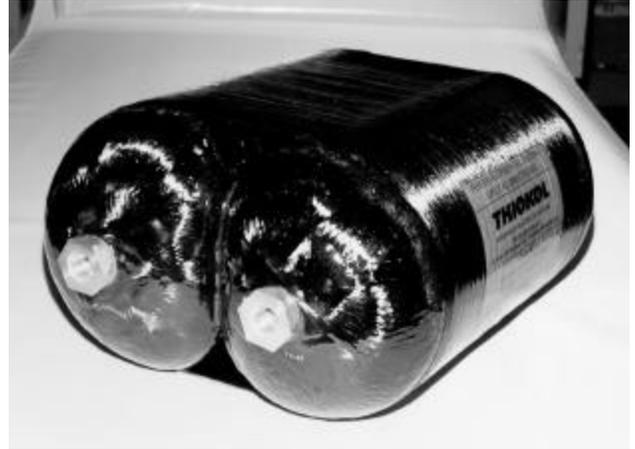
**Figure 3.** Full-scale conformable tank.
