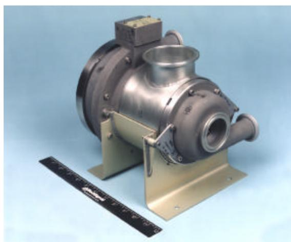
**Figure 1.** Photograph of turbocompressor.
