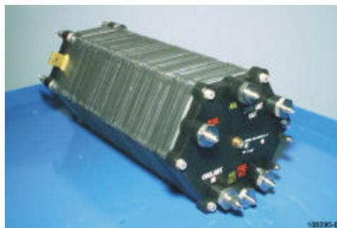
Figure 5. First 10-kW-class stack.
