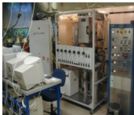
Figure 3. Transient catalytic reactor capable of simulating automotive transients. It can change the gas composition and flow rate instantaneously and can raise the catalyst temperature to 1100°C in < 30 s.
