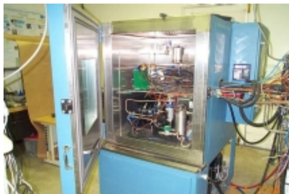
Figure 2. Environmental chamber and apparatus for cold-start measurements.
