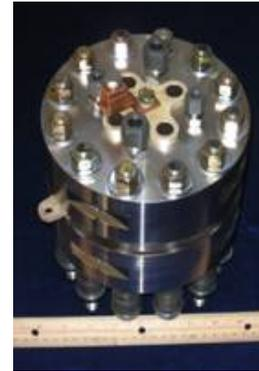
**Solid State Hydrogen Compressor (EHC)**
