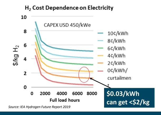
Today's hydrogen cost from PEM electrolyzers: ~ \$5 to \$6/kg at \$0.05 to \$0.07/kWh
