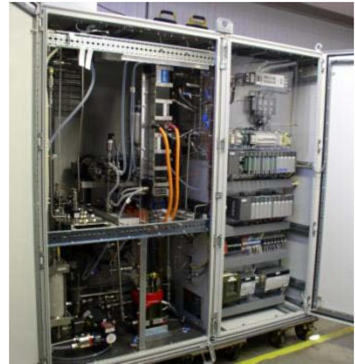
Proton's closed loop RFC system on test, demonstrating feasibility of UUV power concept
