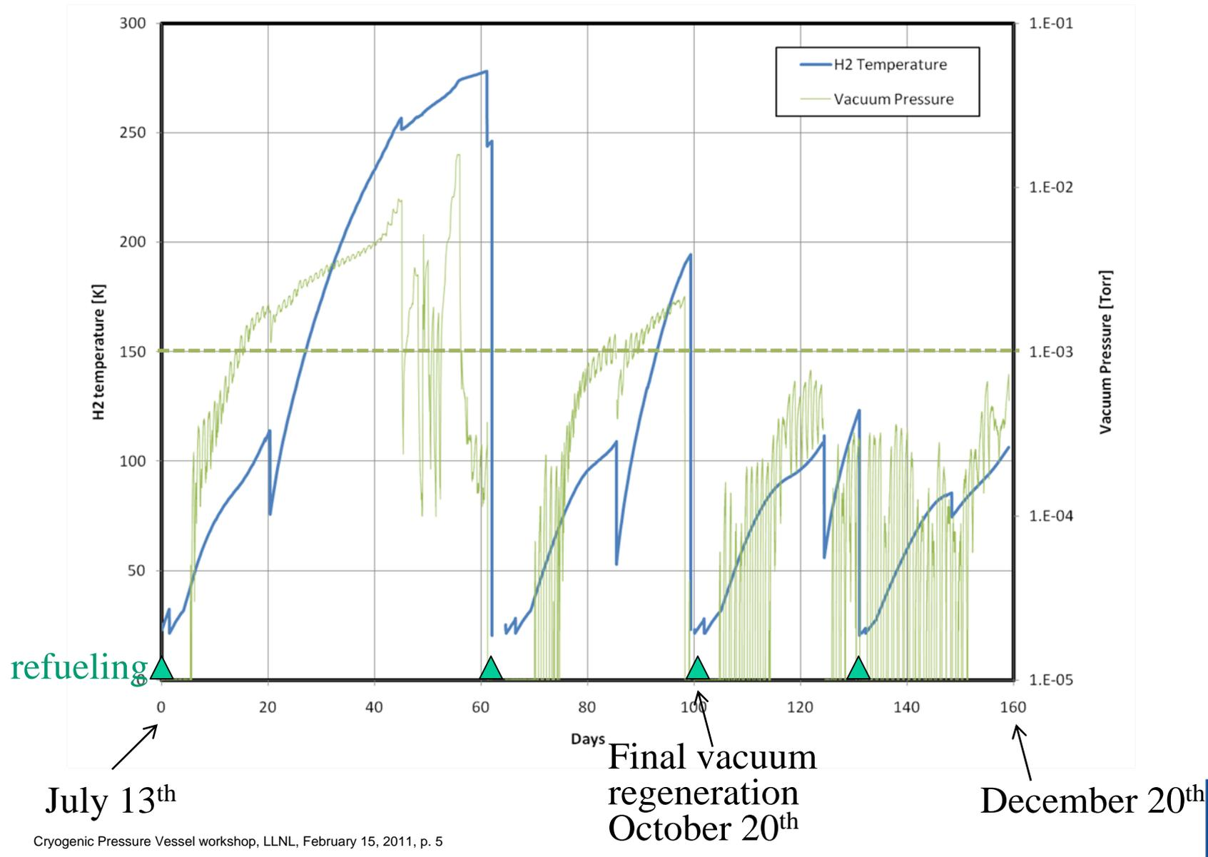
**Para-ortho conversion became significant at ~75 K and extended dormancy by ~5 days for 70-90% full 151 L vessel**
