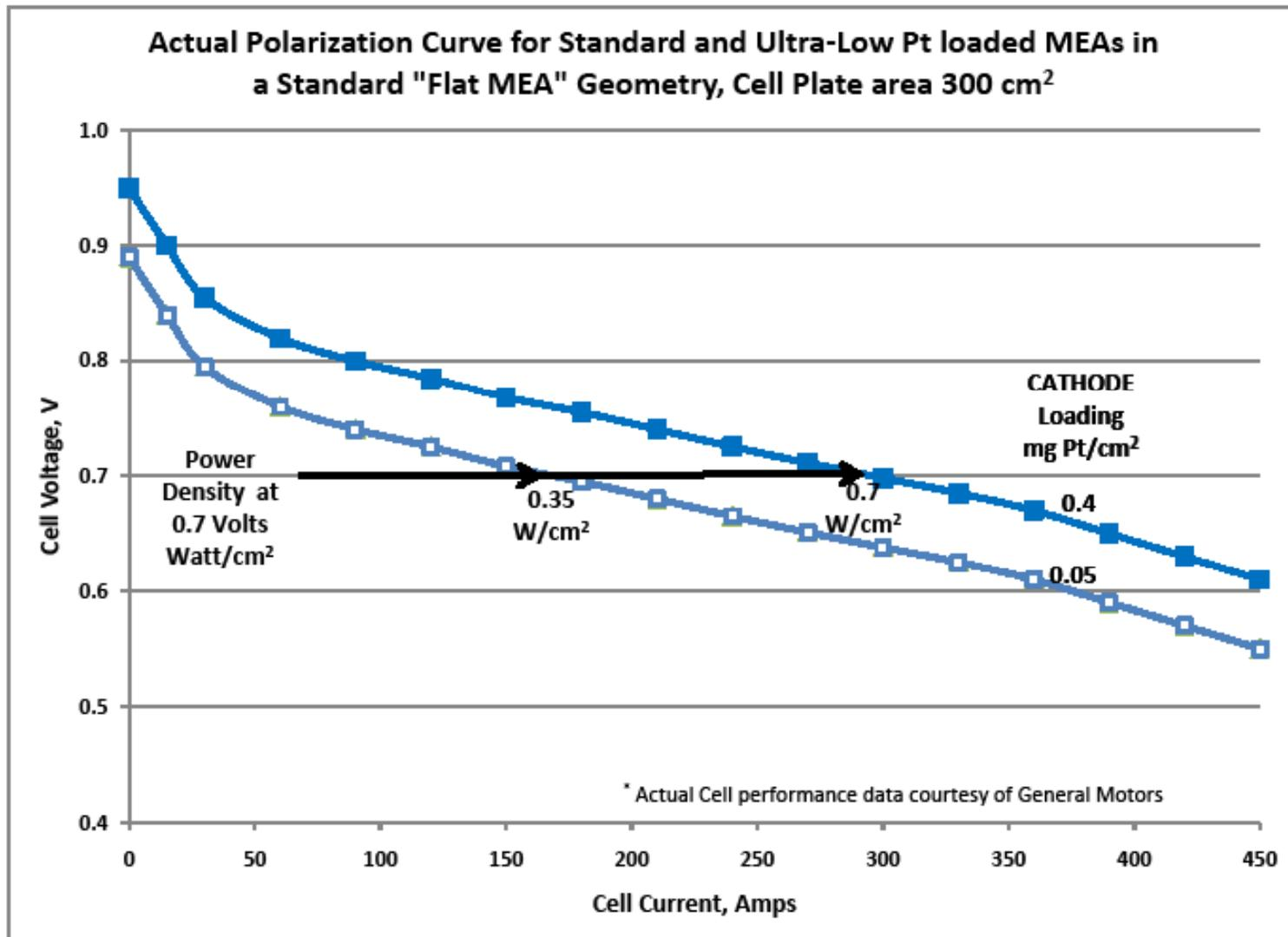
Take-Away: Low Pt loaded MEAs have good Pt Utilization (kW/g Pt) but suffer from low power density (W/cm<sup>2</sup>) thus don't reduce stack costs (Read current state of the art)
