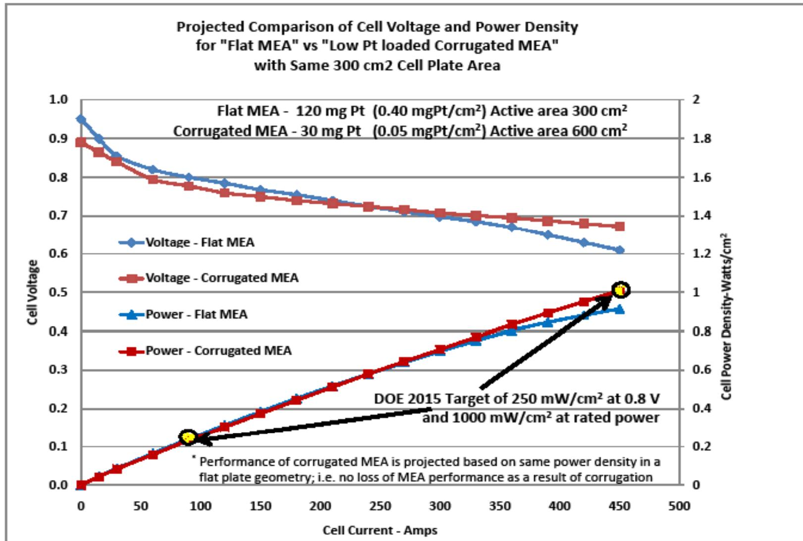
Take-Away: If low Pt loaded MEA is built in the "Corrugated MEA" configuration, it achieves the DOE Power Density targets of 250 mW/cm<sup>2</sup> and 1000 mW/cm<sup>2</sup> at low and rated power.
