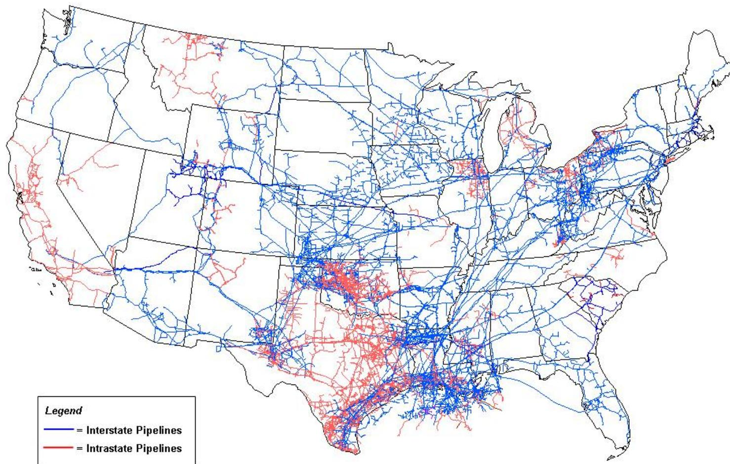
**Figure 6. U.S. natural gas pipeline network in 2009 (EIA 2012).**
