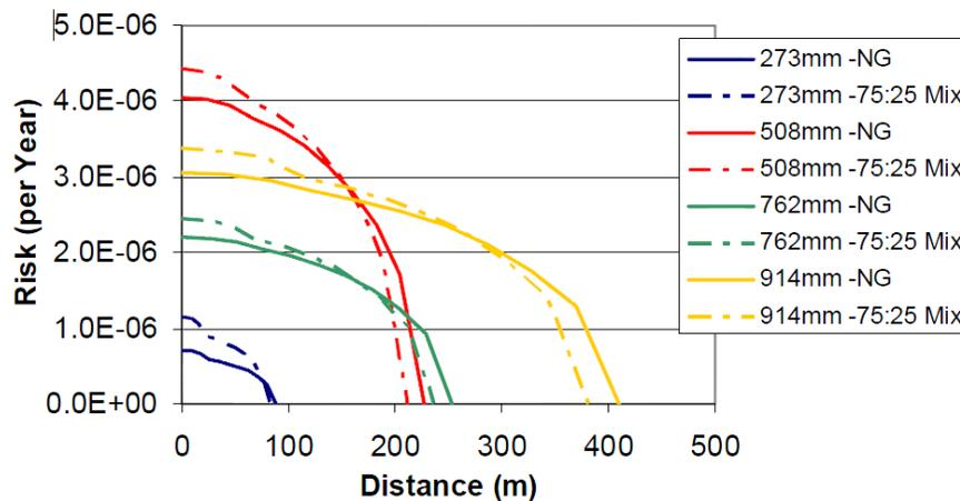
**Figure 13. Risk to an individual per year by adding hydrogen to the natural gas pipeline: UK data.**
