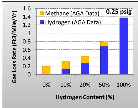
**Figure 9. The Calculated Gas Loss Rate vs. Hydrogen Concentration in Hydrogen/Methane Mixtures at the Typical Distribution Operating Pressures (60 psig (4.1 bar), 3 psig (210 mbar) and 0.25 psig (17.2 mbar))\***
