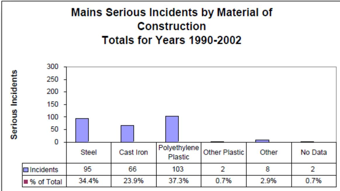
**Figure 7. Serious Incidents by Construction Materials of Mains\***
