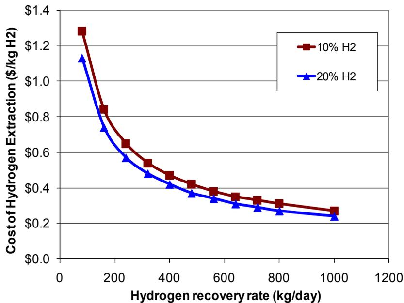
**Figure 18. Estimated cost of hydrogen extraction by PSA unit at the pressure-reduction facility (from 300 psi to 30 psi).**
