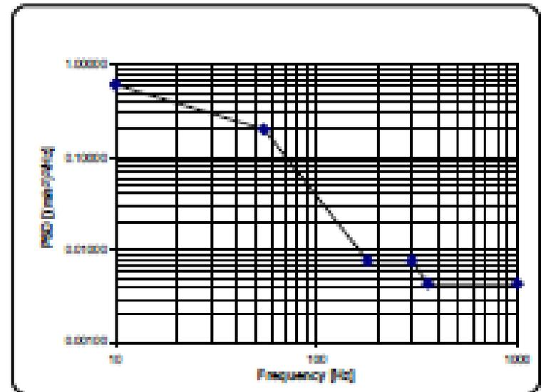
Effective Acceleration =  $4.9 \text{ m/s}^2 = 0.5 \text{ G}_{\text{RMS}}$
