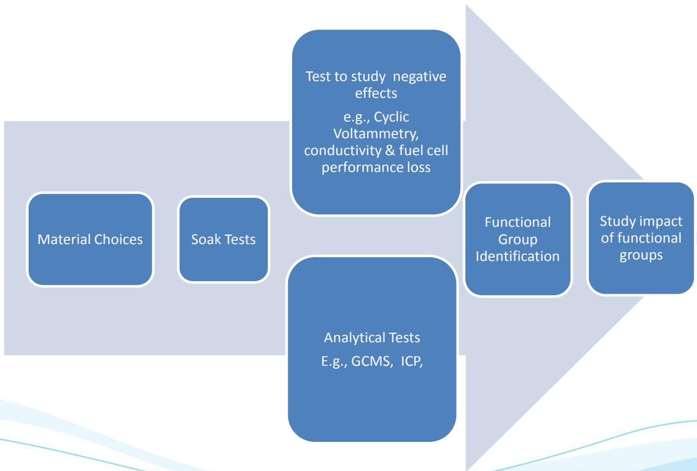
Tests planned to identify functional groups and understand impact on Fuel Cell Durability
