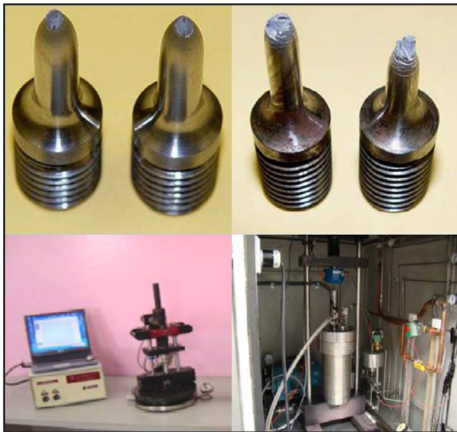
Test Sample Failures (LHS Cup & Cone RHS Faceted Surface) and High Pressure Test Equipment
