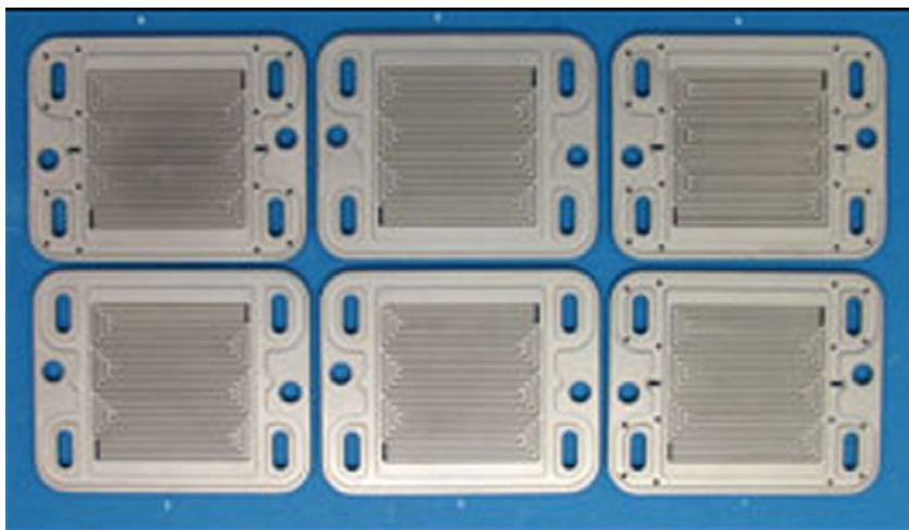
ORNL's Nitrided Metallic Bipolar Plates (Produced in collaboration with DANA Corporation, Tennessee Technological University, and the University of South Carolina)
