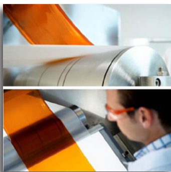
BASF's Roll Membrane Manufacturing Process
