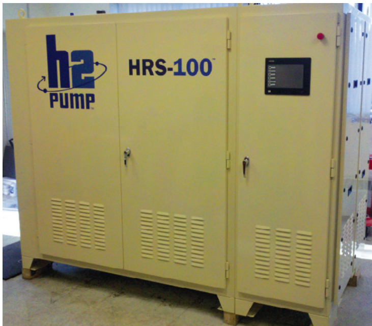
H2Pump's 100 kg/day Hydrogen Recycling System
