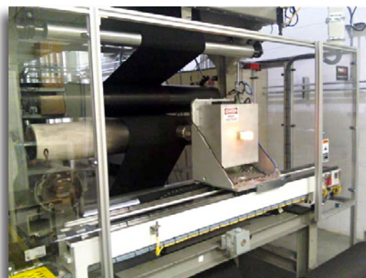
BASF’s High-Speed Coating Machine with XRF Monitoring
