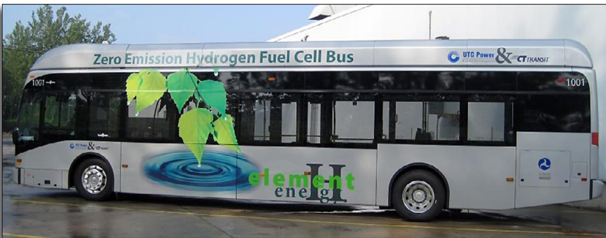
Next Generation CT TRANSIT Fuel Cell Bus powered by the PureMotion Model 120 FCPP
