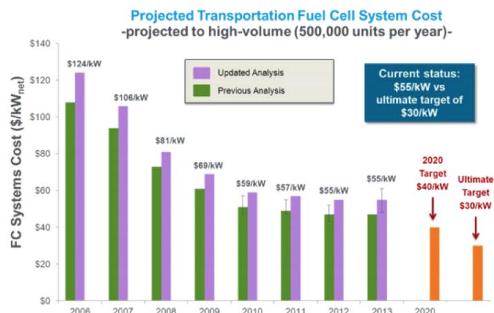
Figure 22: DOE's EERE Fuel Cell Technologies Office Transport Fuel Cell System Cost Status and Targets
