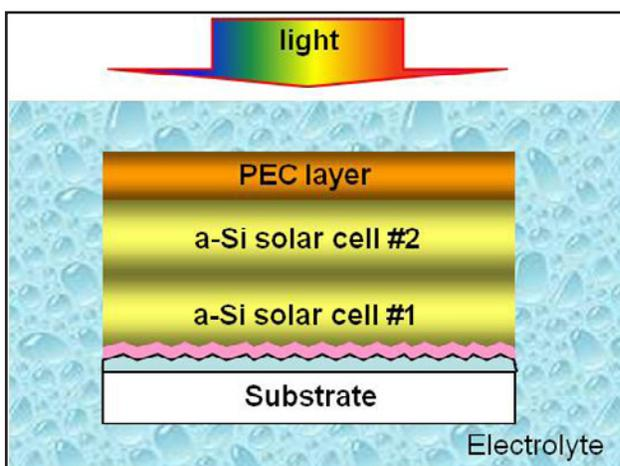
MVSystems' Monolithic Hybrid PEC Device Powered By a Tandem Solar Cell
