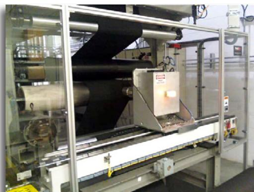
*BASF's High-Speed Coating Machine with XRF Monitoring*
