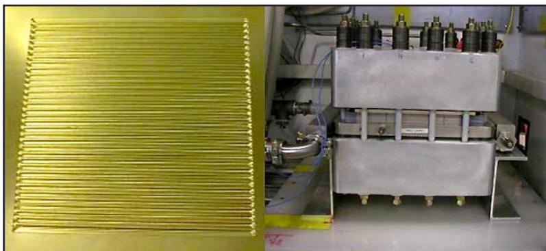
Proton's Consolidated Bipolar Plate and 0.6 ft<sup>2</sup> Electrolysis Stack (right)
