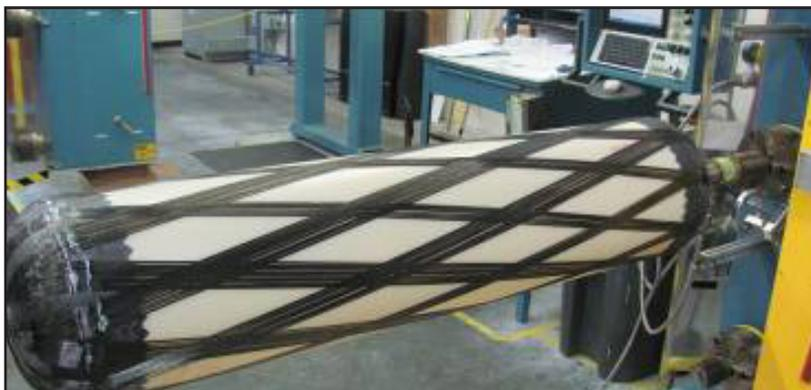
*Quantum's Hybrid Manufacturing Technology for Pressure Vessels*
