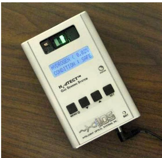
*IOS's Prototype H<sub>2</sub>-dTECT Hydrogen Sensor*
