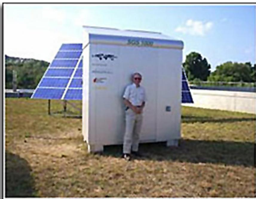
*The Avalence Electrolysis Unit with Photovoltaic Array*
