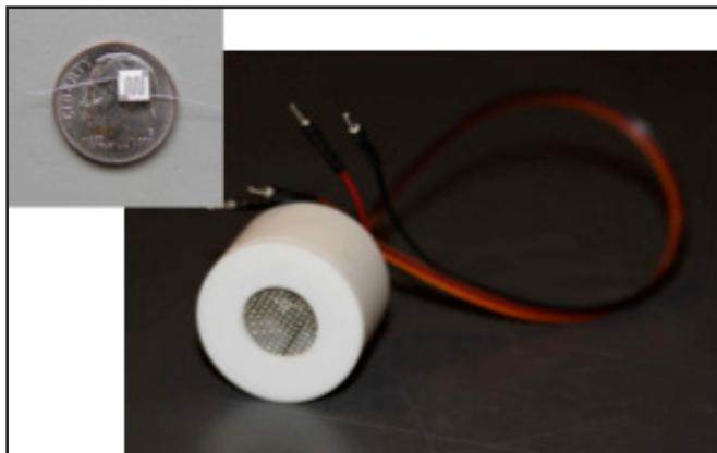
*Packaged Electrochemical H<sub>2</sub> Safety Sensor*
