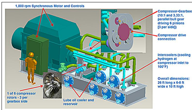
Concepts NREC's Centrifugal Hydrogen Pipeline Gas Compressor
