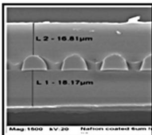
Micrographs of Giner's Dimensionally Stable Membrane
