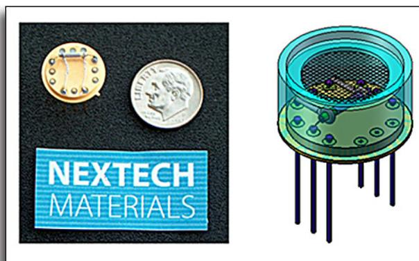
*Ceramic Sensor Element used in the SenseH<sub>2</sub>*
