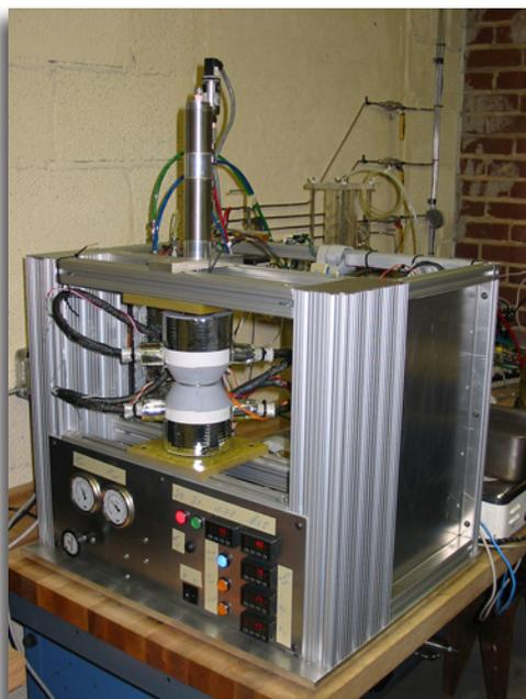
*Scribner Associates' Rapid Membrane Measurement System Prototype*
