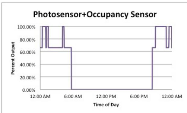
**Figure 13.** Monitoring for the same structure using both photo and occupancy sensor controls. When daylight is available, the luminaire is off. When it is dark outside, the luminaire is controlled by the occupancy sensor.
