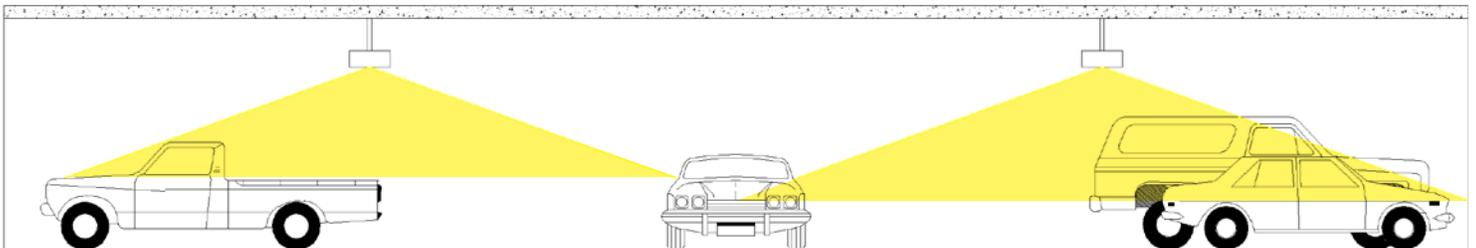
**Figure 7.** Double luminaire layout.
