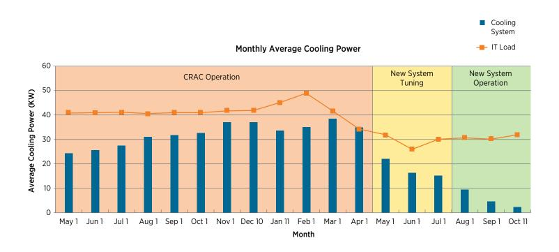
Figure 5. Monthly average cooling power comparison between CRAC system and new system.
