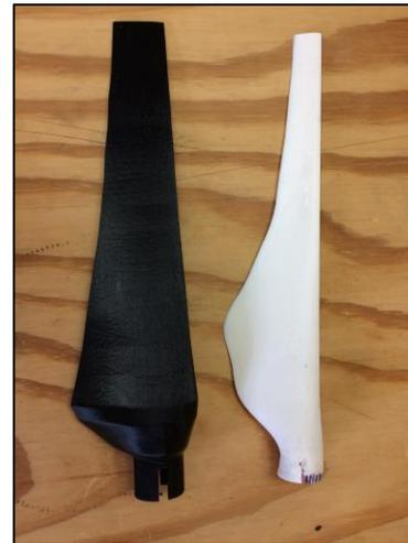
**Figure 18:** Comparison of first generation (right) and second generation blades (left)
