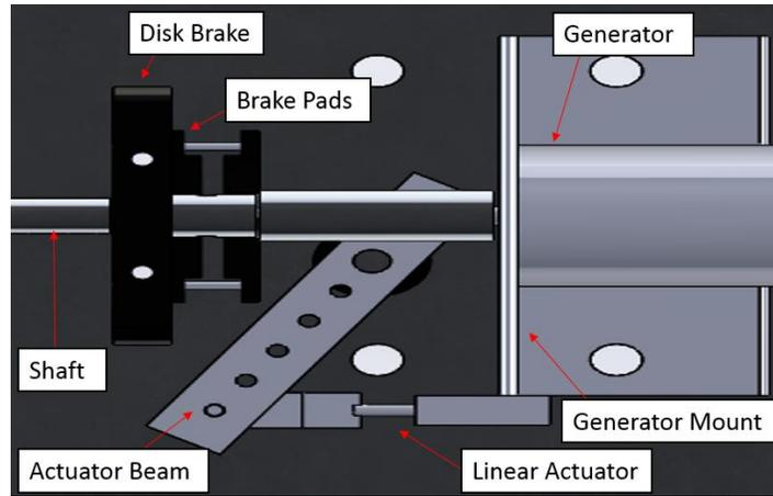
Figure 7: Disk Brake Assembly
