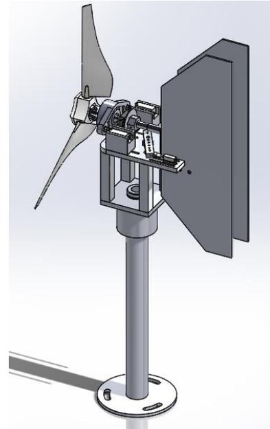
Figure 3: SolidWorks Model of Tunnel Turbine
