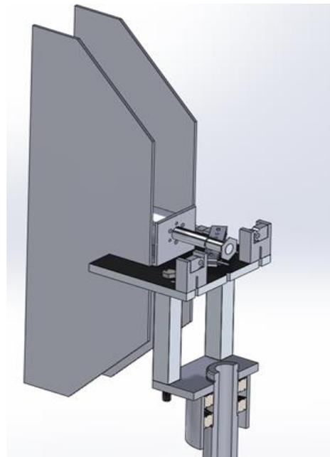
Figure 10: Section View of Bearing Sleeve Yaw system.
