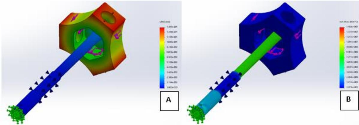
Figure 6: SolidWorks FEA: Hub displacement (A) and von Mises Stress (B).
