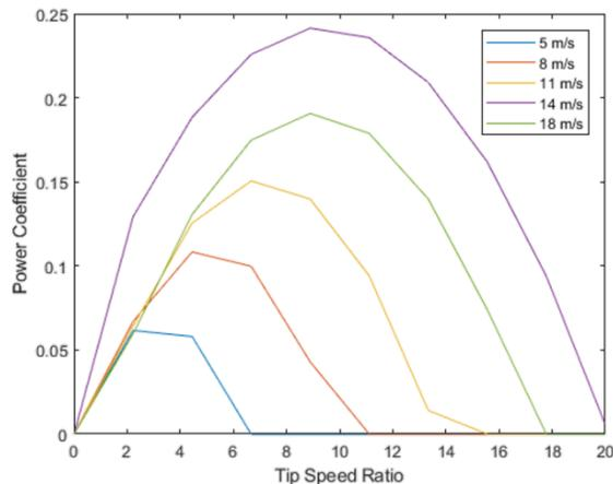
Figure 4: Power Coefficient vs. Tip-Speed Ratio
