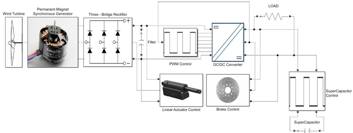
Figure 11: Tunnel Turbine Electrical System
