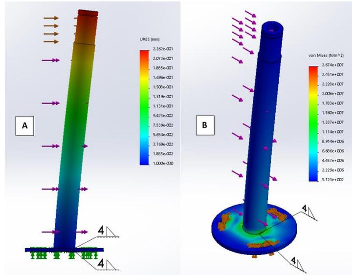
Figure 9: SolidWorks FEA: Tower Displacement (A) and von Mises Stress (B).
