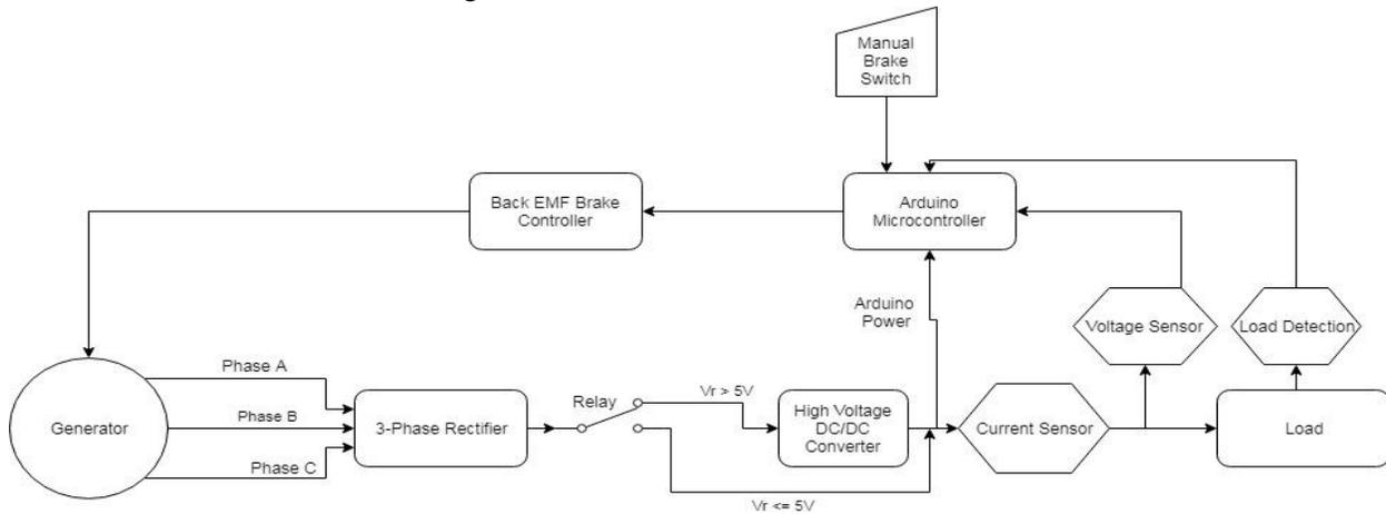
Figure 23. Box diagram showing power flow
