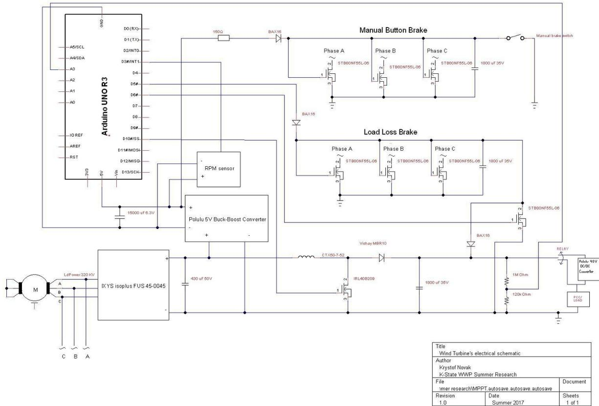
Figure 22. Test turbine circuit schematic
