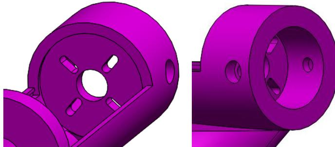
Figure 9. Generator and tail connection to the back of the nacelle
