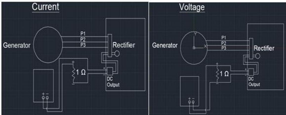
Figure 24. Wiring diagram for test set up
