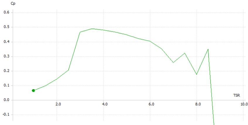
Figure 5. Test turbine Qblade graph for 5 blades
