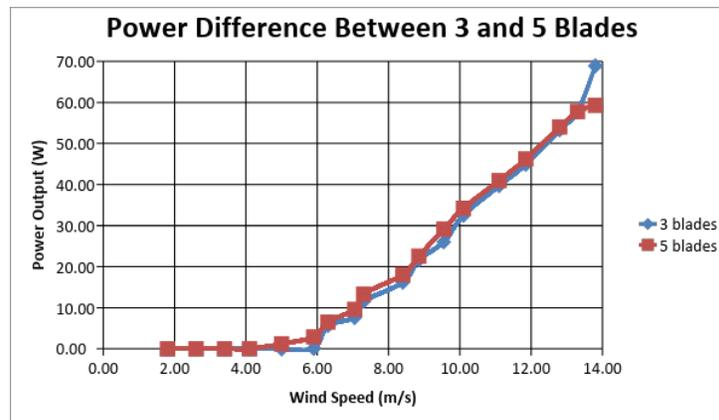
Figure 16. Graph of the power difference between three and five blades
