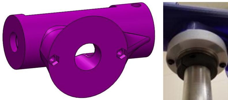
Figure 8. Tower connection to bottom of the nacelle
