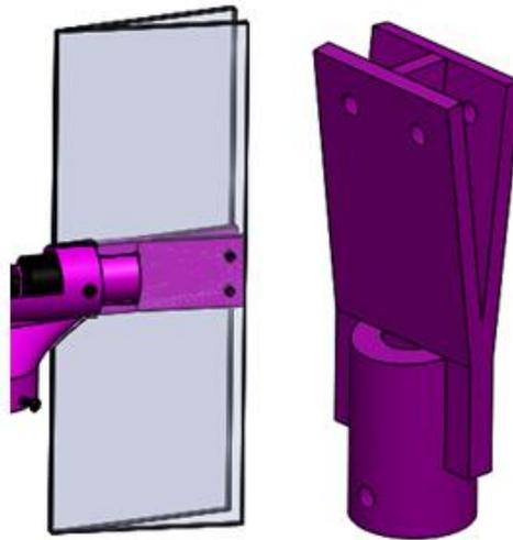
Figure 15. Twin-wing tail and adapter
