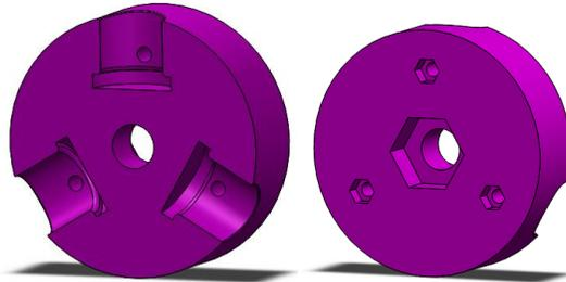
Figure 17. Nut side of the fixed pitch hub
