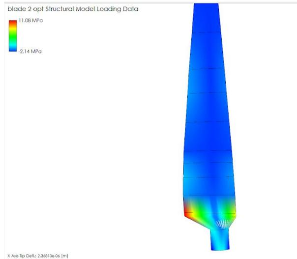
Figure 7. QBlade FEA analysis for twisted blades at TSR of 4
