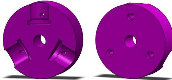
Figure 18. Screw side of the fixed pitch hub
