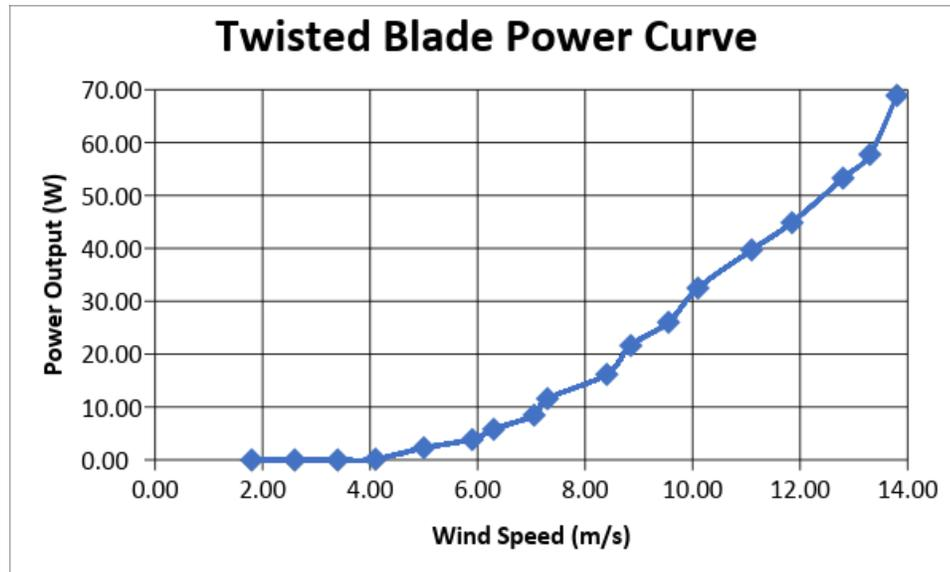
Figure 25. Twisted blade power curve
