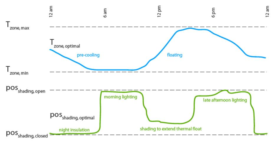
**Challenge:** Determine shading position and radiant cooling level to minimize energy consumption for lighting and cooling over a 24-h period, subject to zone temperature constraints and given weather forecast. Overlay TOU rates and on-site BIPV/ storage source availability for energy cost minimization.
