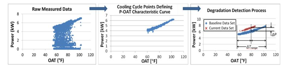
**Degradation is detected when**  $\Delta P > \Delta P_{alarm threshold}$
