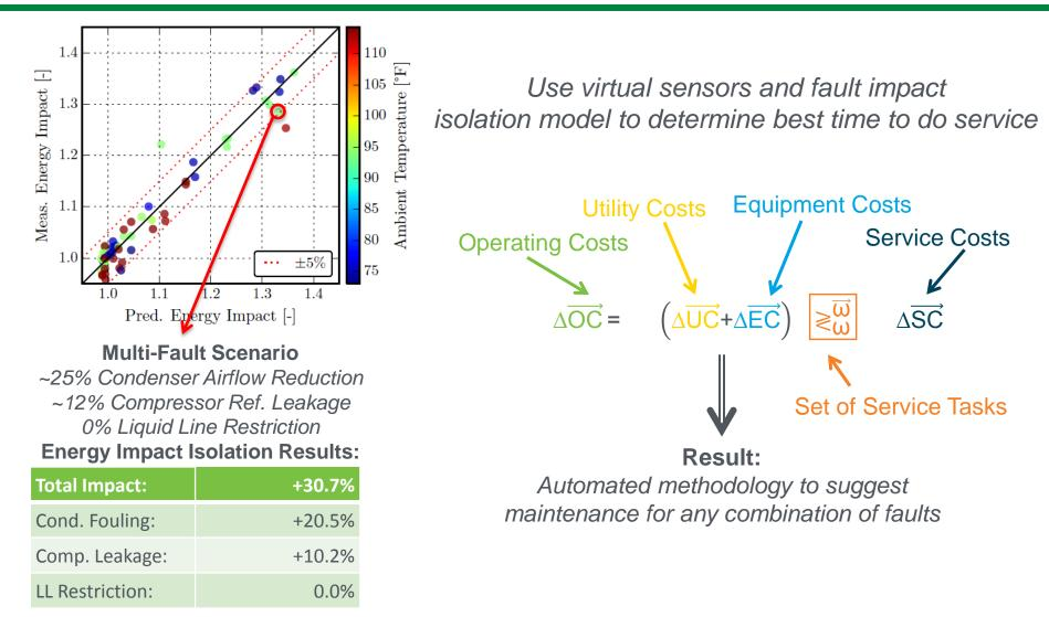
Methodology for fault ranking and service decision making developed
