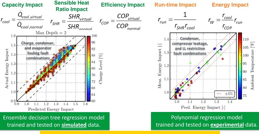
Model for fault energy impact evaluation developed
