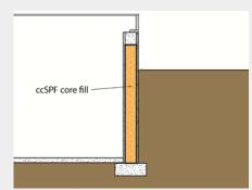
**Step 1.** Hollow masonry block cores are filled with ccSPF to block convection currents and associated moisture transfer.
