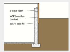
**Step 3.** 2 in. of exterior rigid foam is added down to 1 ft below grade to control heat loss and warm interior surface temperatures.
