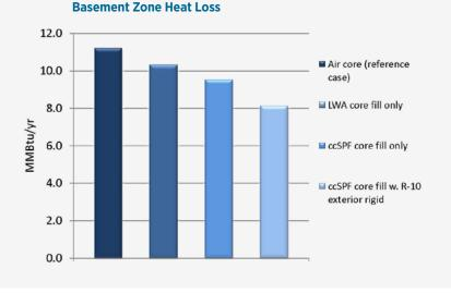
A simple ccSPF core fill reduced basement zone heat loss by 15%. Combining a ccSPF core fill with R-10 exterior rigid insulation installed to 1 ft below grade reduced heat loss by 27%.
