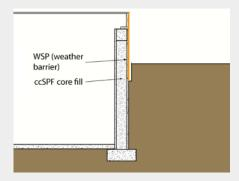
**Step 2.** A water-control layer is added to the exterior rim joist down to 1 ft below grade to shed bulk water.
