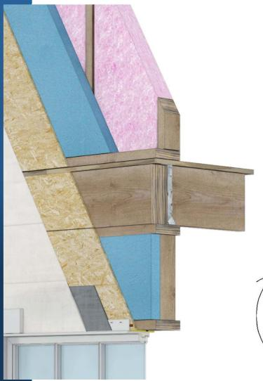
Header built into the floor
