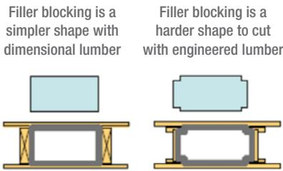
Wood or rigid foam filler blocking is needed to close off the gaps between floor joists to form an air break between conditioned and unconditioned spaces.
