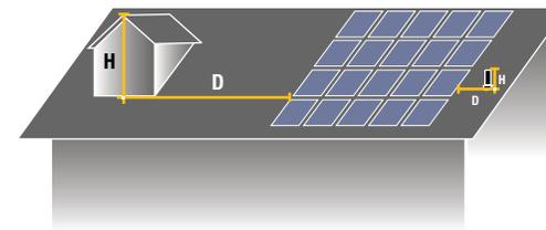
For houses with solar photovoltaic roof panels, any potential shading structure should be twice as far away from the PV array as it is tall ( $D = 2 * H$ )
