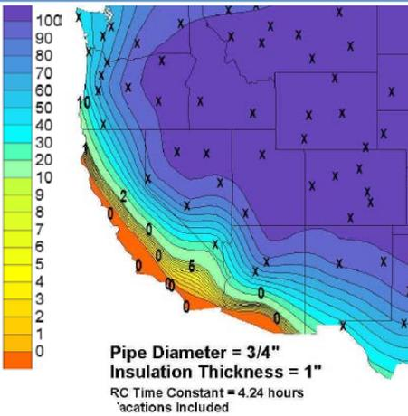
Integrated Collector Storage solar water heating systems are well suited to areas with little threat of freezing such as most of the California coast and southern Arizona. Other types of solar thermal water heaters are available including flat-plate collectors in indirect systems that use antifreeze; these systems work well in areas where freezing temperatures are possible. (Figure source: Jay Burch of NREL)
