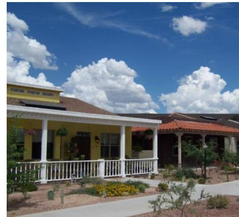
Deep overhangs and porches help minimize heat gain to the interior of the home. Xeriscaping minimizes irrigation needs in the hot dry climate.
