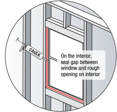
On the interior, seal gap between window and rough opening on interior
