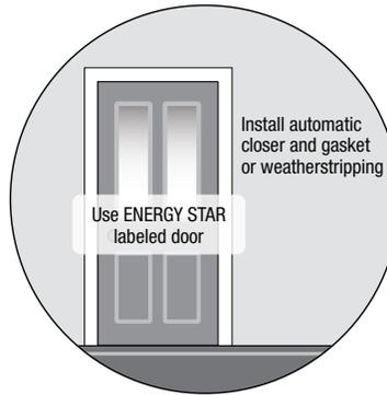
Install automatic closer and gasket or weatherstripping
