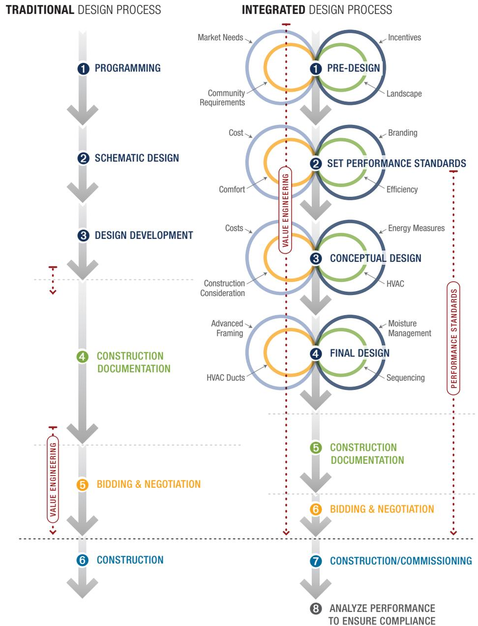
The Integrated Design Process loops in design input at every stage of development. (Adapted from IEA 2003)
