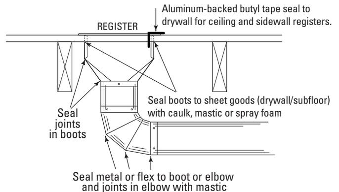
Mastic is a goeey adhesive that is applied wet. It fills gaps and dries to a soft solid. Mastics may or may not contain reinforcing fibers, and they may be used with reinforcing mesh tape.
