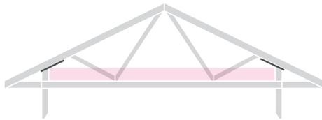
Raised heel trusses allow space for the full depth of insulation. Dark lines are baffles which allow ventilation of roof while keeping wind from blowing back insulation.
