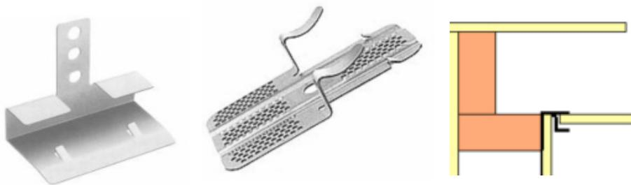
Two-stud corners with drywall clips use the least wood and give the best thermal performance.
