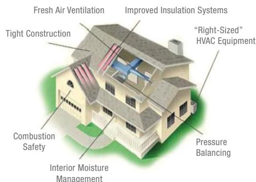
Pulte Las Vegas takes a systems approach with its homes that combines advanced framing, increased insulation, and improved air sealing with right-sized HVAC, mechanical ventilation, transfer grilles, and jump ducts for lower utility bills and guaranteed comfort. (Figure source: Pulte Las Vegas)
