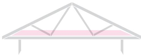
Traditional roof trusses pinch insulation where the roof meets the walls
