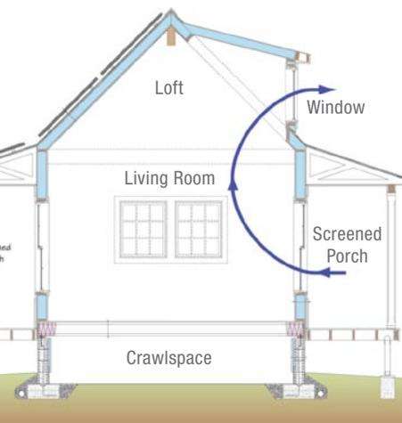
Building America's Building Science Consortium used convection to help cool this structural insulated panel (SIPs) cottage in Georgia. Cool air from the screened porches is drawn into the building's interior where it heats up and is pulled up and out the second-story windows, drawing more air in through the shaded first-story windows.
