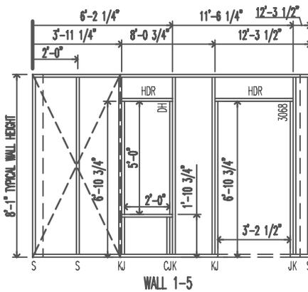
Provide framing diagrams to spell out advanced framing techniques.
