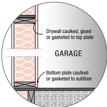
Drywall caulked, glued or gasketed to top plate
