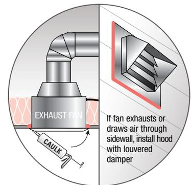
If fan exhausts or draws air through sidewall, install hood with louvered damper
