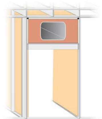
**5** Drywallers finish exposed surfaces with sealed, caulked, taped, and mudded drywall and seal connection of duct boot to drywall.
