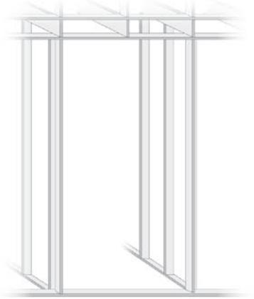
**2** Install drywall or OSB or other air barrier extending past the area to be included in chase. Framers may install gypsum board.
