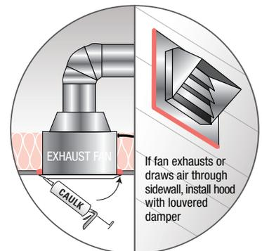
Provide bathroom and kitchen exhaust fans. Duct them to the outside and caulk ducts at the dry wall for an air-tight seal. Use low speed fans for quiet operation.
