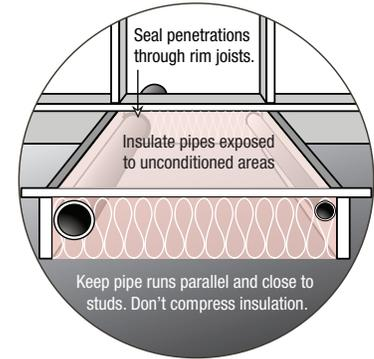
Seal penetrations through rim joists.
