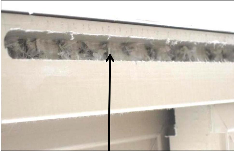
Improperly cut orifice
