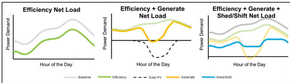
**Figure 4. Daily Average Load Profiles for a Grid-interactive Efficient Building<sup>17</sup>**
