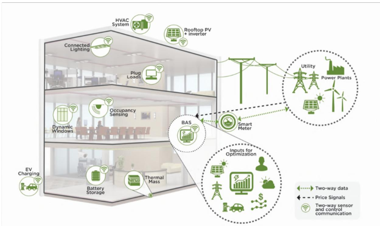
**Figure 2. Example Commercial Grid-interactive Efficient Building<sup>5</sup>**
