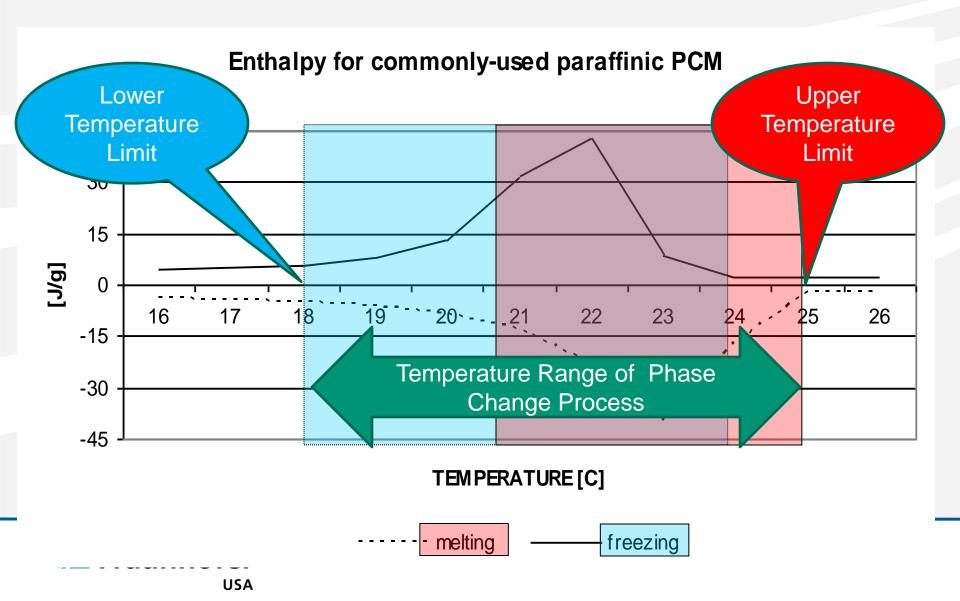
Example of estimation of temperature ranges for DHMA
