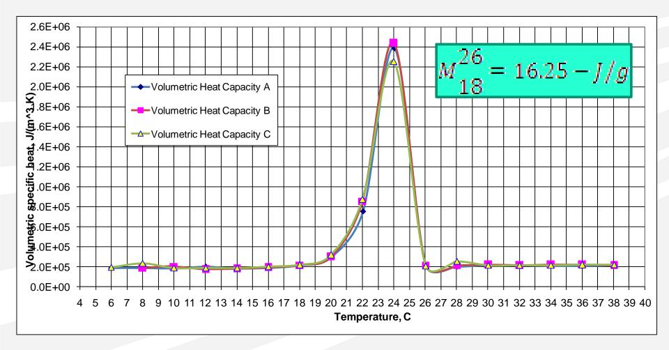
Described above measurements yielded the total enthalpy of the tested PCM-enhanced material of 16.25 J/g, with a +/-3.4% difference between the highest and lowest results.
