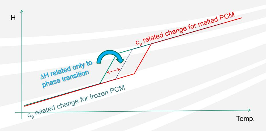
It is possible to analytically estimate and later subtract  $c_p$ -related enthalpy changes for both frozen and melted stages of the testing.
