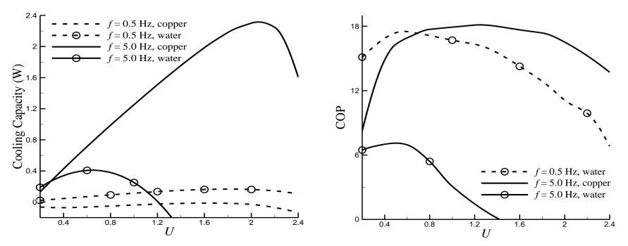
Cooling Capacity (left) and COP (right) as a function of utilization with f = 0.5 and 5.0 Hz
