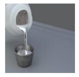
Galinstan is a metal that is in liquid phase at room temperature.
