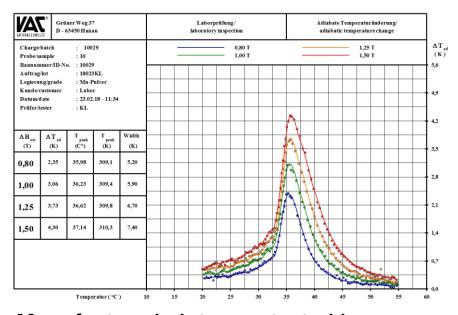
Manufactured plate was tested in calorimeter to characterize its magnetocaloric effect. The graph shows that it retained its magnetic properties.
