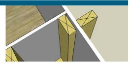
Offsetting the interior wall framing from the exterior wall framing allows drywall to be slid between the two rather than stopping at each corner so the drywall can form a continuous air barrier along the exterior wall.
