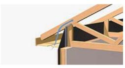
When OSB or plywood wall sheathing is extended up the wall, it provides adequate support for raised heel trusses so no extra blocking is needed. The sheathing also serves as an insulation baffle.
