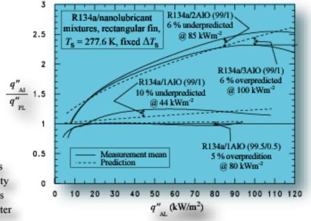
The model and the measurements agreed to within 10 % for all of the data with heat fluxes less than 100 kWm<sup>-2</sup>.
