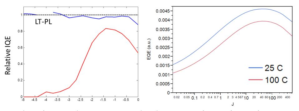
Peak IQE (measured using Low Temp Photoluminescence) = **85**% (407 nm) Current droop (measured using Electroluminescence) = **97**% Thermal droop (measured using High Temp Electroluminescence) = **85**% (to 100 °C)
