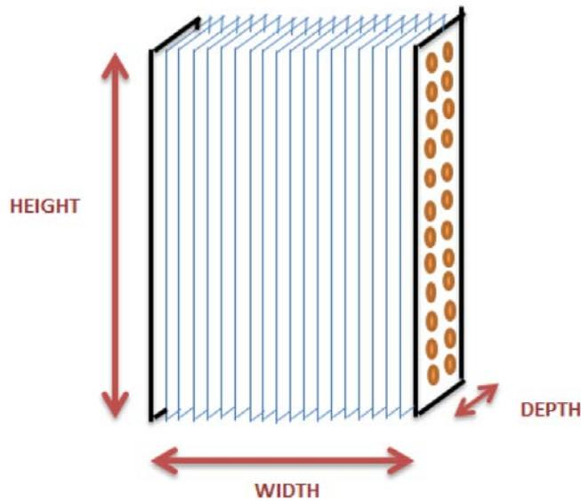
Figure 1: Evaporator Coil Dimensions
