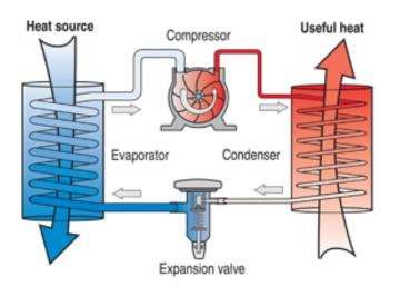
Condenser: High-temperature heat exchanger where the refrigerant enters as a high-temperature vapor, rejects heat to the heat sink by condensation at a high pressure and leaves as a high-temperature liquid.
