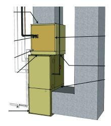
Standard 193 encourages manufacturers to install gaskets and take other steps to minimize air leaks in furnace cabinets. (Figure source: Calcs Plus 2014)
