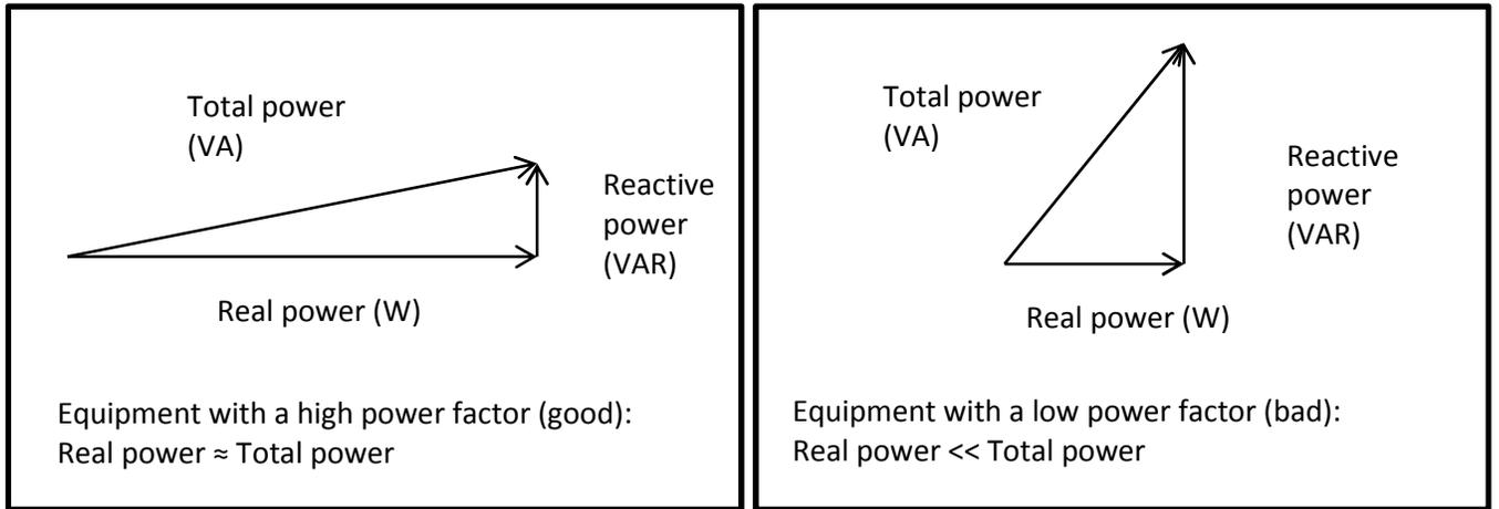
**Figure D.2: Comparison of Power Factor for Different Equipment**
