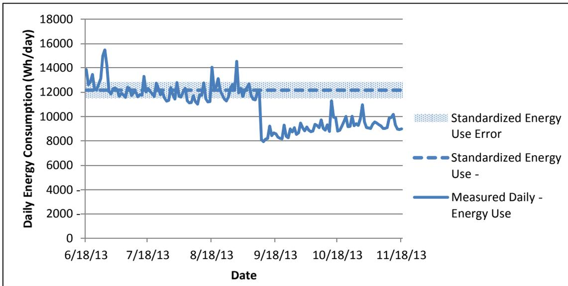
**Figure B.3: Unadjusted Measured Daily Energy Use v. Standardized Daily Energy Use: Unit Demo-2**
