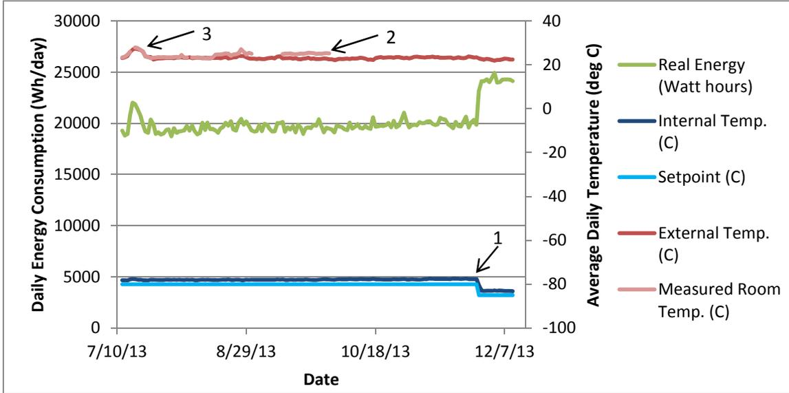
**Figure A.11: Daily Energy and Temperature Data: Unit Comp-3**
