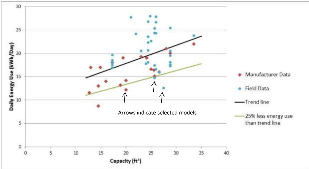
**Figure II.1 Graph of Available ULT Energy Data with Selected Models Indicated\***
