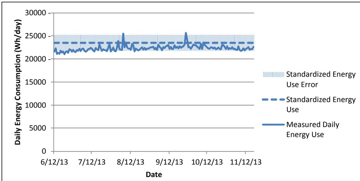
**Figure B.2: Unadjusted Measured Daily Energy Use v. Standardized Daily Energy Use: Unit Comp-1**
