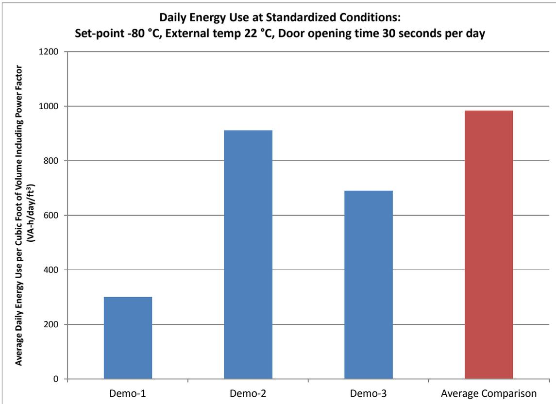
**Figure III.3: Adjusted Electricity Consumption for Demo and Average Comparison ULTs, Accounting for Power Factor\***
