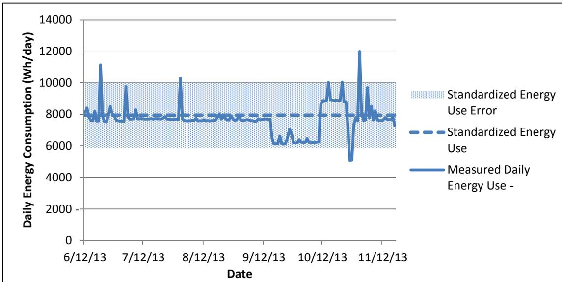
**Figure B.1: Unadjusted Measured Daily Energy Use v. Standardized Daily Energy Use: Unit Demo-1**
