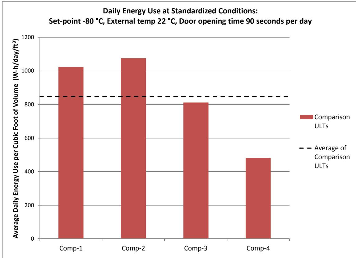
**Figure III.2: Adjusted Daily Energy Consumption for Comparison ULTs without Space Conditioning Impacts**
