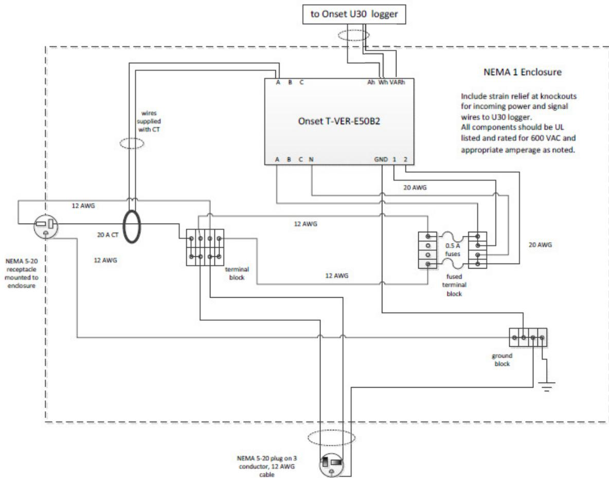
Figure C.1: Electrical Diagram for NEMA 5-20 Connector
