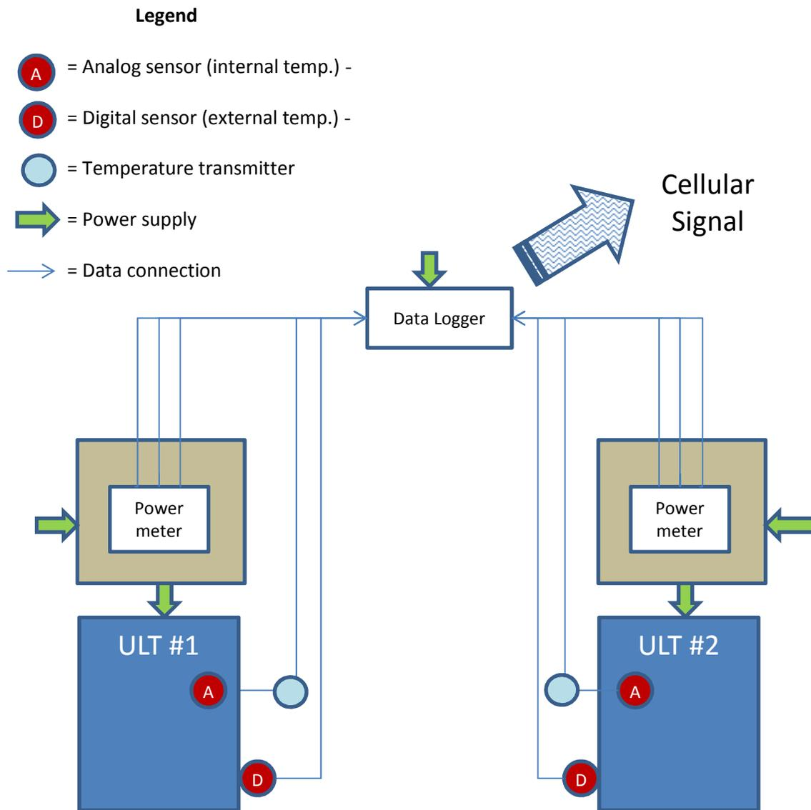
**Figure C.11: Instrumentation Schematic for CU Boulder Sites**
