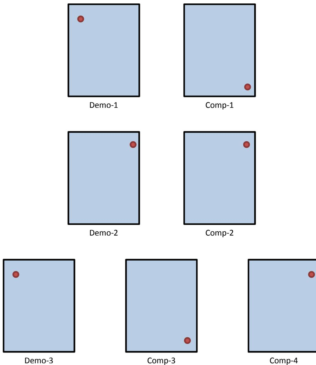
**Figure C.5: Front View of Each ULT Showing Approximate Relative Elevation of Internal Thermocouple Placement**
