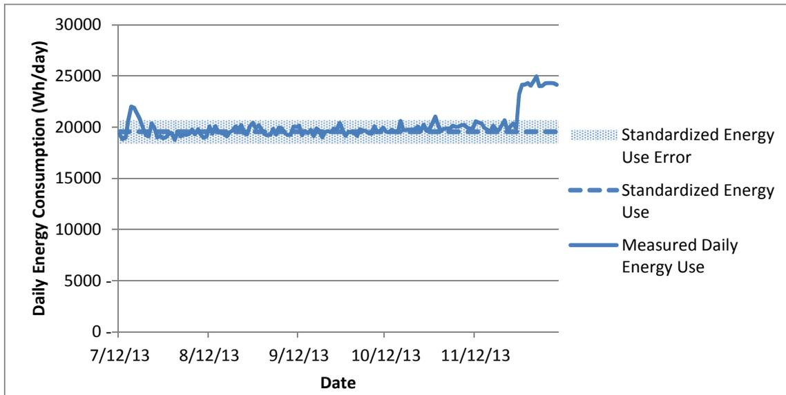
**Figure B.6: Unadjusted Measured Daily Energy Use v. Standardized Daily Energy Use: Unit Comp-3**
