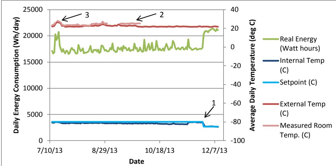
**Figure A.9: Daily Energy and Temperature Data: Unit Demo-3**
