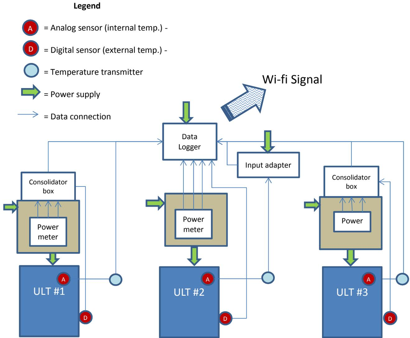
**Figure C.12: Instrumentation Schematic for Michigan State University Lab**
