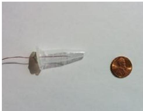
(2) Thermocouple embedded in vial
