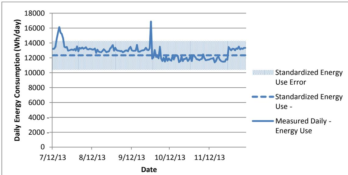
**Figure B.7: Unadjusted Measured Daily Energy Use v. Standardized Daily Energy Use: Unit Comp-4**
