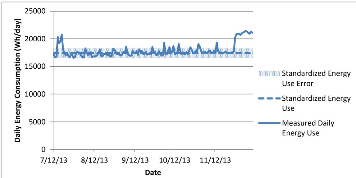
**Figure B.5: Unadjusted Measured Daily Energy Use v. Standardized Daily Energy Use: Unit Demo-3**
