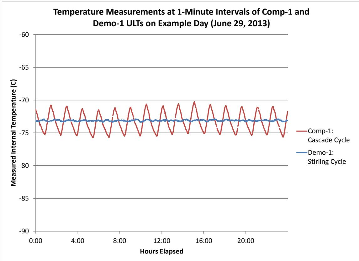
**Figure III.5: Comparing Internal Temperature of Cascade and Stirling Cycle ULTs**
