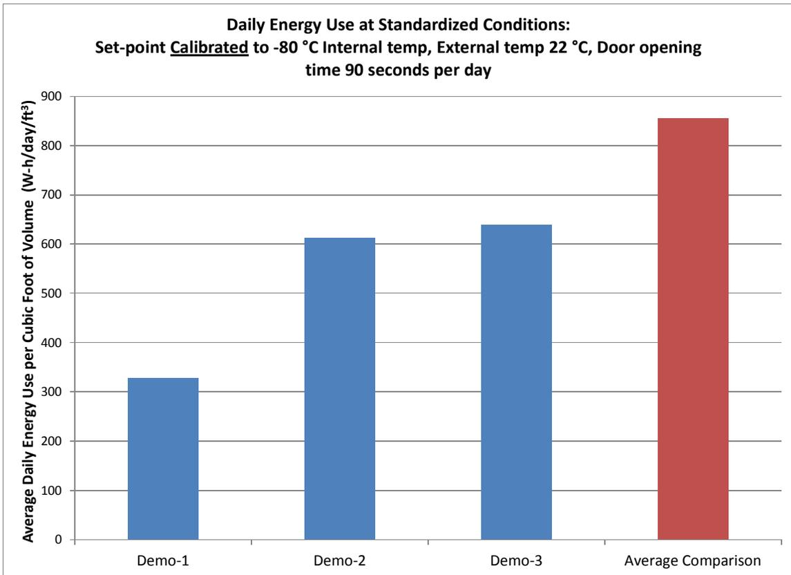
**Figure III.4: Adjusted Electricity Consumption for Demo and Average Comparison ULTs, Calibrating Set-Point to Internal Temperature of -80 °C\***
