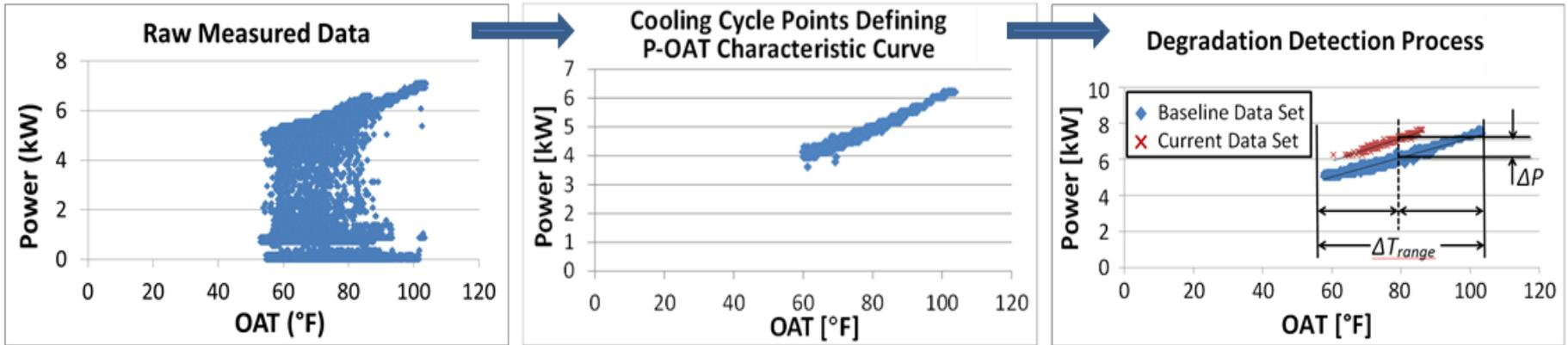
Degradation is detected when  $\Delta P > \Delta P_{alarm\ threshold}$
