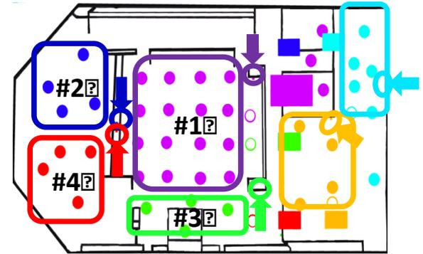
○ thermostat ● supply diffuser ■ RTU
