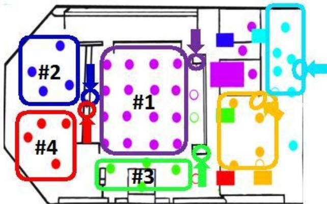
○ thermostat ● supply diffuser ■ RTU
