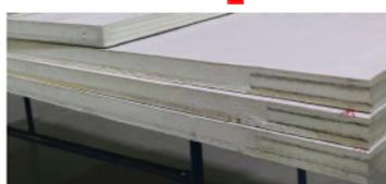
Finished composite insulation boards
