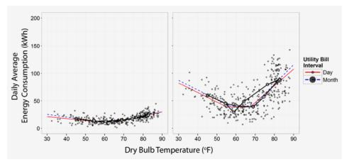
The above image illustrates the differences between the measured energy consumption of two homes. The overlaid inverse modeling results quantify in simple terms the differences between the homes and allow for comparison on more terms than simply total annual energy consumption. Note how the models with monthly resolution inputs (solid red lines) closely align with the daily (dashed blue lines). Good-quality monthly data are adequate for simple weather normalization using linear models.
