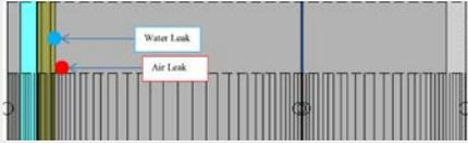
Double stud wall with cellulose insulation and polyethylene vapor retarder
