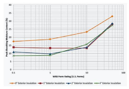
The graph above shows that the exterior moisture content depends greatly on the permeance of the WRB. A high permeance WRB, regardless of the amount of exterior insulation, will result in dangerously (i.e., 28% MC) high moisture levels in the wood-based sheathing. Exterior insulation, and WRB permeances less than 10 U.S. perms, are highly recommended.
