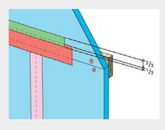
**BEST** — Butyl Z-flashing with 2 in. acrylic termination tape
