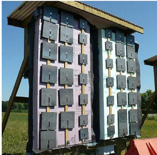
Exterior environmental exposure testing examined four types of insulation materials. Each test panel was constructed with two layers of 2-in. thick insulation and loaded to three different load magnitudes (8 pounds [lbs], 15 lbs, and 30 lbs per fastener). Researchers recorded the downward and upward vertical movement of the furring strips over a period of about 70 days. Daily movements were on the order of  $\pm 1/2$  of an inch.
