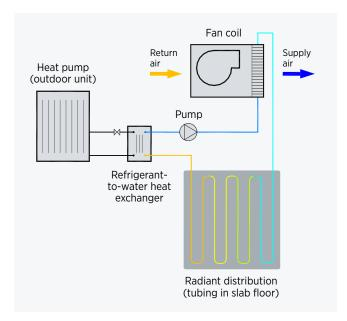
This schematic shows the AWHP system in cooling mode with mixed-mode distribution. In cooling mode, the refrigerant-towater heat exchanger acts as the evaporator. Chilled water first circulates through a fan coil, which supplies latent cooling to the house and raises the temperature of the supply water to the radiant floor. Most sensible cooling is then distributed through tubes embedded in the radiant slab floor.
