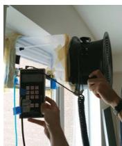
Apparatus for testing airflow through a trickle vent (left) and actual test in progress (right).
